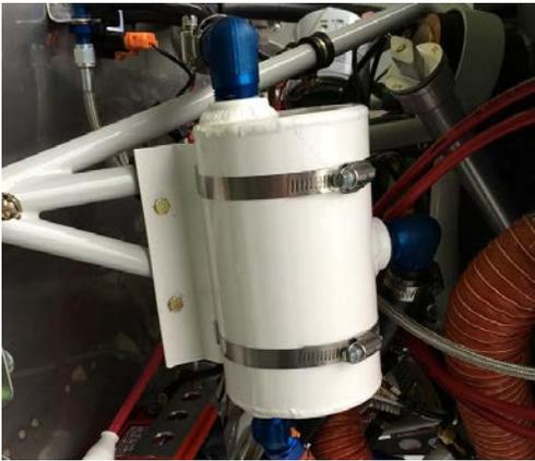
The inverted oil system consists of an inverted/upright shuttle valve, an oil/air separator canister and a system of interconnecting lines. Oil pressure may be interrupted momentarily in certain aircraft attitudes or during certain combinations of maneuvers. These interruptions are normal but should not be allowed to extend beyond 15 seconds (avoid extended right knife edge flight).
