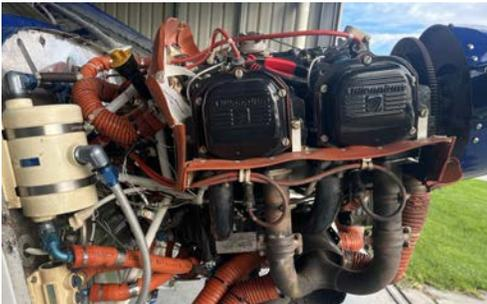
The Super Decathlon is equipped with a **Lycoming AEIO-360-H1B**, 4-cylinder, fuel injected engine rated at 180 horsepower at 2700 RPM. The engine is direct drive, air cooled, and naturally aspirated. Engine ignition is provided by two engine driven magnetos which are independent of each other and the aircraft's electrical system.
