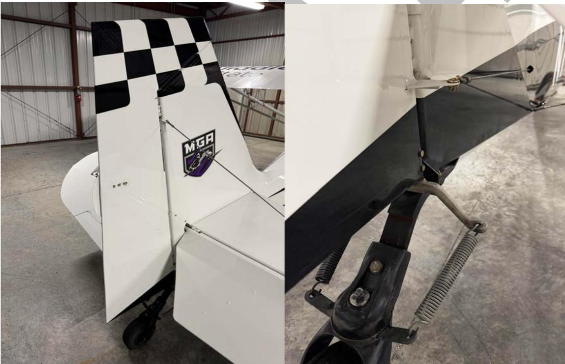
The rudders control yaw about the vertical axis and are connected via cables and pulleys. Unlike a tricycle gear airplane, the tailwheel is connected to the rudder via springs rather than direct linkages. This reduces “shimmy” on taxi and takeoff roll but can make taxi and turning more challenging. To make more precise turns, pilots should utilize differential braking of the main gear. Additionally, unlike nose-gear, tailwheels can caster 360 degrees, allowing for better turning radius.
