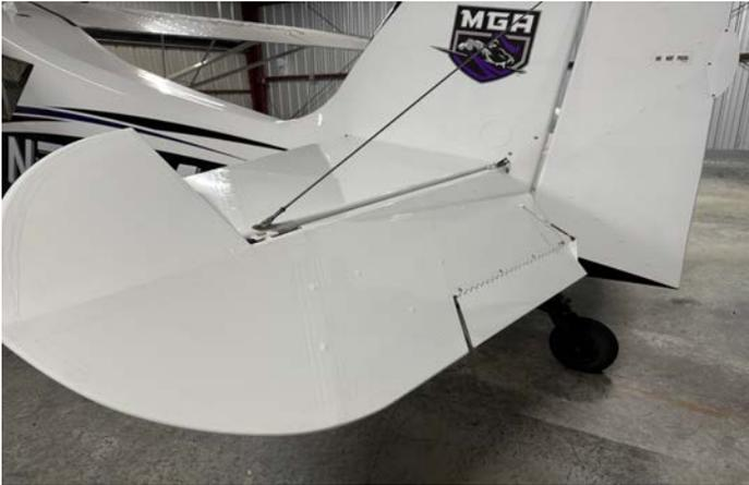
The elevator controls aircraft pitch about the lateral axis. Unlike the stabilator of most Piper aircraft, both the Super Decathlon and Citabria have a traditional separate horizontal stabilizer and elevator.
