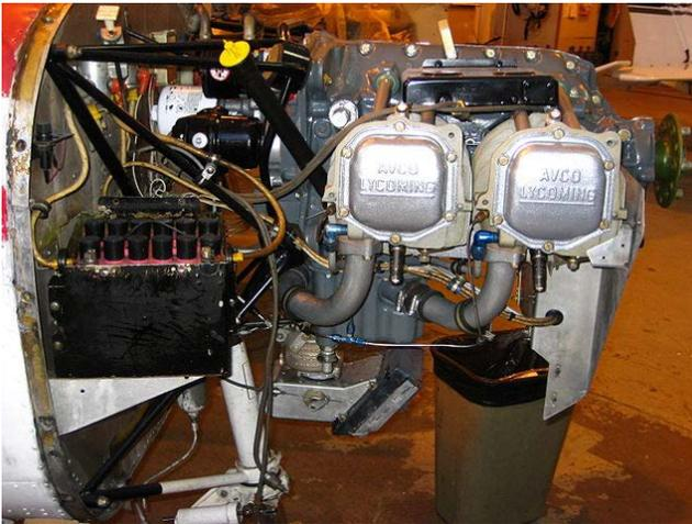
The Citabria is equipped with a **Lycoming O-235-K2C**, 4-cylinder, carbureted engine rated at 115 horsepower at 2700 RPM. The engine is direct drive, air cooled, naturally aspirated, and has a wet-sump oil system. Engine ignition is provided by two engine driven magnetos which are independent of each other and the aircraft's electrical system.
