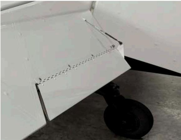
Both the Super Decathlon and Citabria have traditional trim tabs. Unlike a balance tab or anti-servo tab, traditional trim tabs are static, meaning their angle relative to the elevator doesn't change with elevator deflection.
