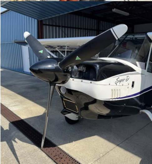
The Super Decathlon is equipped with an MT-Propeller, manufactured by MT-Propeller Entwicklung GmbH, a German company renowned for its advanced propeller designs. These propellers feature a natural composite construction, utilizing multilaminate spruce and compressed plastified beech wood (also known as "Superwood"). The wooden core is reinforced with carbon fiber composite and protected by a Nickel-Cobalt erosion sheet, providing durability and performance.
