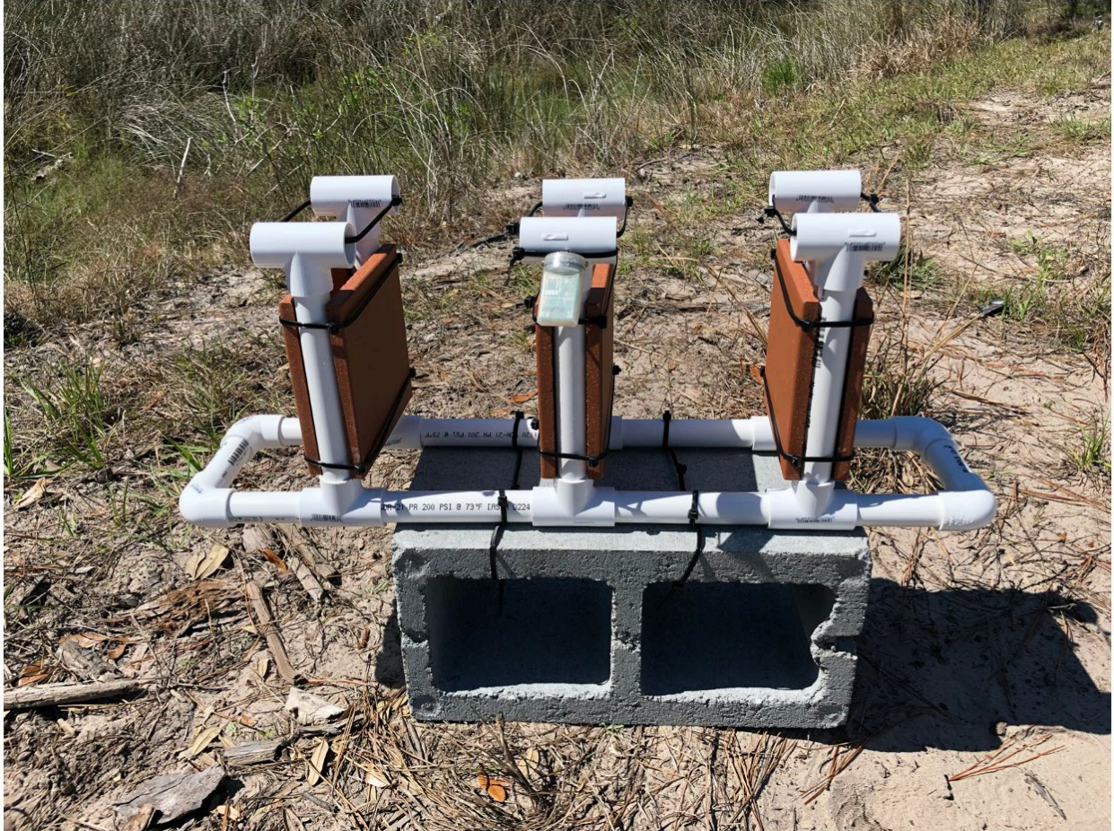
Figure 3. Oyster spat rack. Six ceramic tiles measuring 15 X 15 cm were attached to the rack with zip ties.
